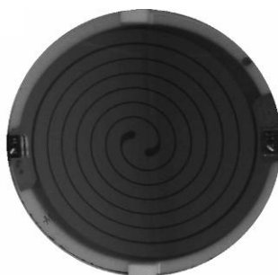
a) Bi-spiral thin film YBCO for resistive current limiter
