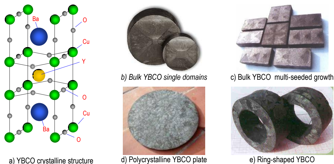
Figure 27 - Ceramic YBCO crystalline structure and the various shapes
