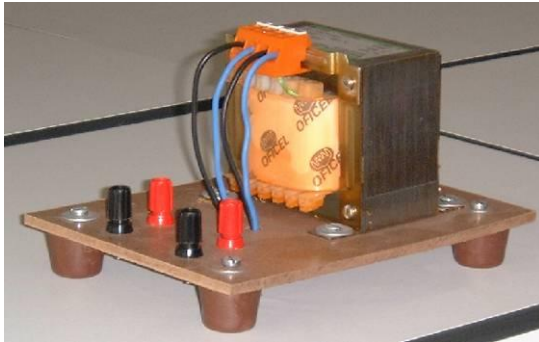
Figure 44 - Experimental transformer with crystalline iron core
